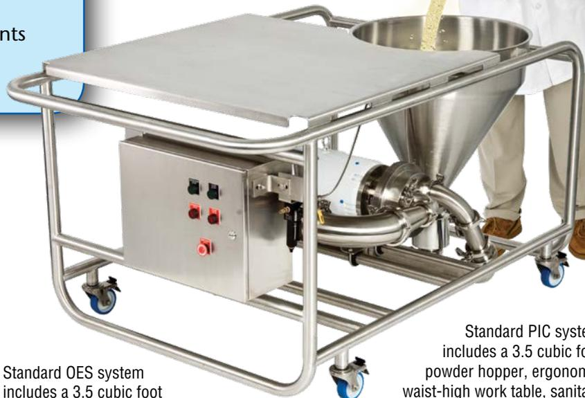
Standard PIC system includes a 3.5 cubic foot powder hopper, ergonomic waist-high work table, sanitary powder suction pump, powder valve, vacuum gauge, vacuum regulator valve, control box for pump and interconnecting piping
