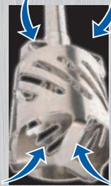
**3.** Centrifugal pressure forces material to the periphery of the stator where it is subjected to further mechanical shear as material passes through the sharpened edges of the expanded slots in the stator.
